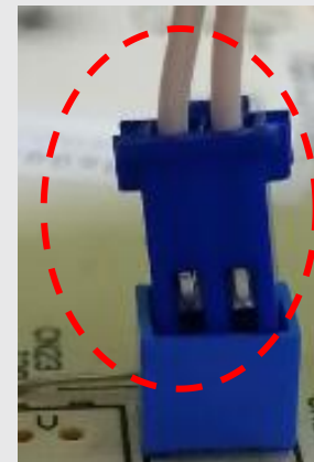
Connector is loose
